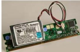
The integrated **ServeRAID-8k-I** controller offers *hardware RAID-0/1/10* support and **32MB** of fast **PC2-4200 DDR2** cache for the SAS drives. The **ServeRAID-8k** option adds **three** additional RAID levels, **RAID-1E, 5** and **6**, along with **256MB** of cache memory for higher performance, and battery backup, *without* consuming a valuable adapter slot.
