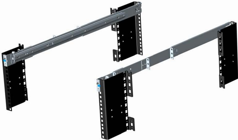
One key factor in selecting the proper rails is identifying the type of rack in which they will be installed. Both the sliding rails and the static rails support tool-less mounting in 19"-wide, EIA-310-E compliant square hole and unthreaded round hole 4-post racks. Both also support tool-ed mounting in threaded hole 4-post racks, but only the static rails, as the more universal solution, support mounting in 2-post (Telco) racks.
