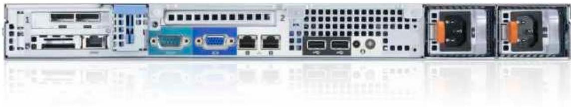
The chassis design of the R320 is optimized for easy access to components and for airflow for effective and efficient cooling. The R320 supports up to 6 DIMMs, 1 processor, hot-plug redundant power supplies, and many other components and features described in this guide.
