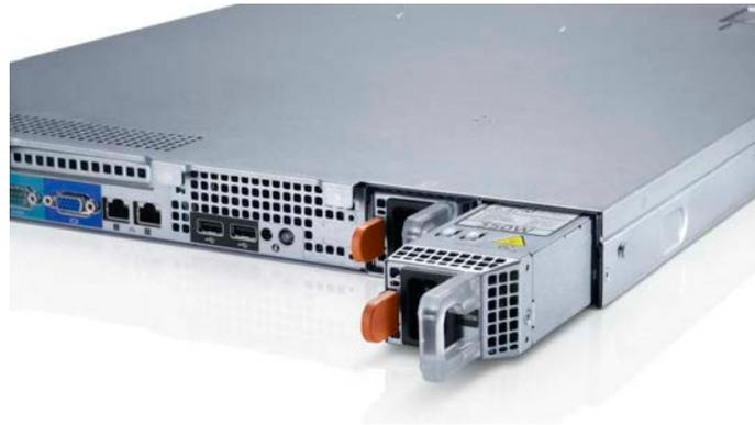
The PowerEdge R320 supports up to two AC with 1+1 redundancy, auto-sensing, and auto-switching capability.
